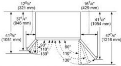
The location must permit both doors to open to a minimum of 90°. Allow 4 1/2" (114 mm) minimum space between the side of the refrigerator and a corner wall.
